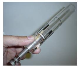
Sample tube depth adjustment: First, seat the spinner on top of the depth gauge. Second, carefully push the sample tube through the spinner holding the tube from the middle (not from top) until the bottom just touches the top of the slider (white
